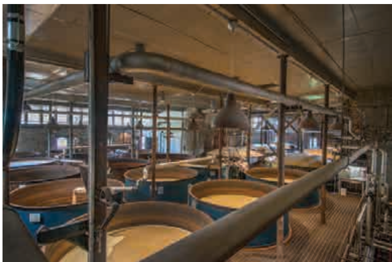
Grain mixes, or mash bills, for whiskeys are fermented before distillation and aging.
